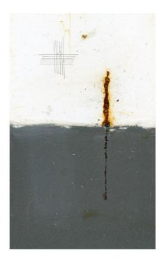
Control vs. a combination of an anticorrosive pigment and a liquid flash rust inhibitor in an APEO free, water based styrene acrylic primer.
