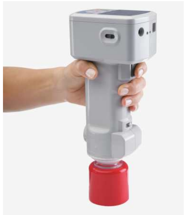
Color measurement of plastic article with spectrophotometer CM-700d (Photo: Konica Minolta)
