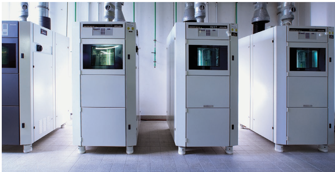
Light exposure for determination of light fastness
